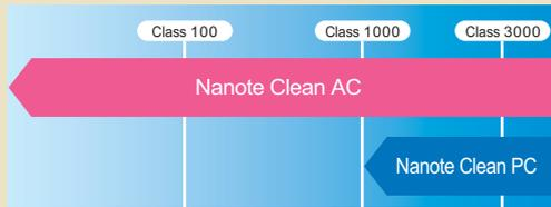
\*Lower class numbers indicate a higher level of clean room cleanliness. Class 100 means no more than 100 particles of 0.5 or more per cubic foot.
